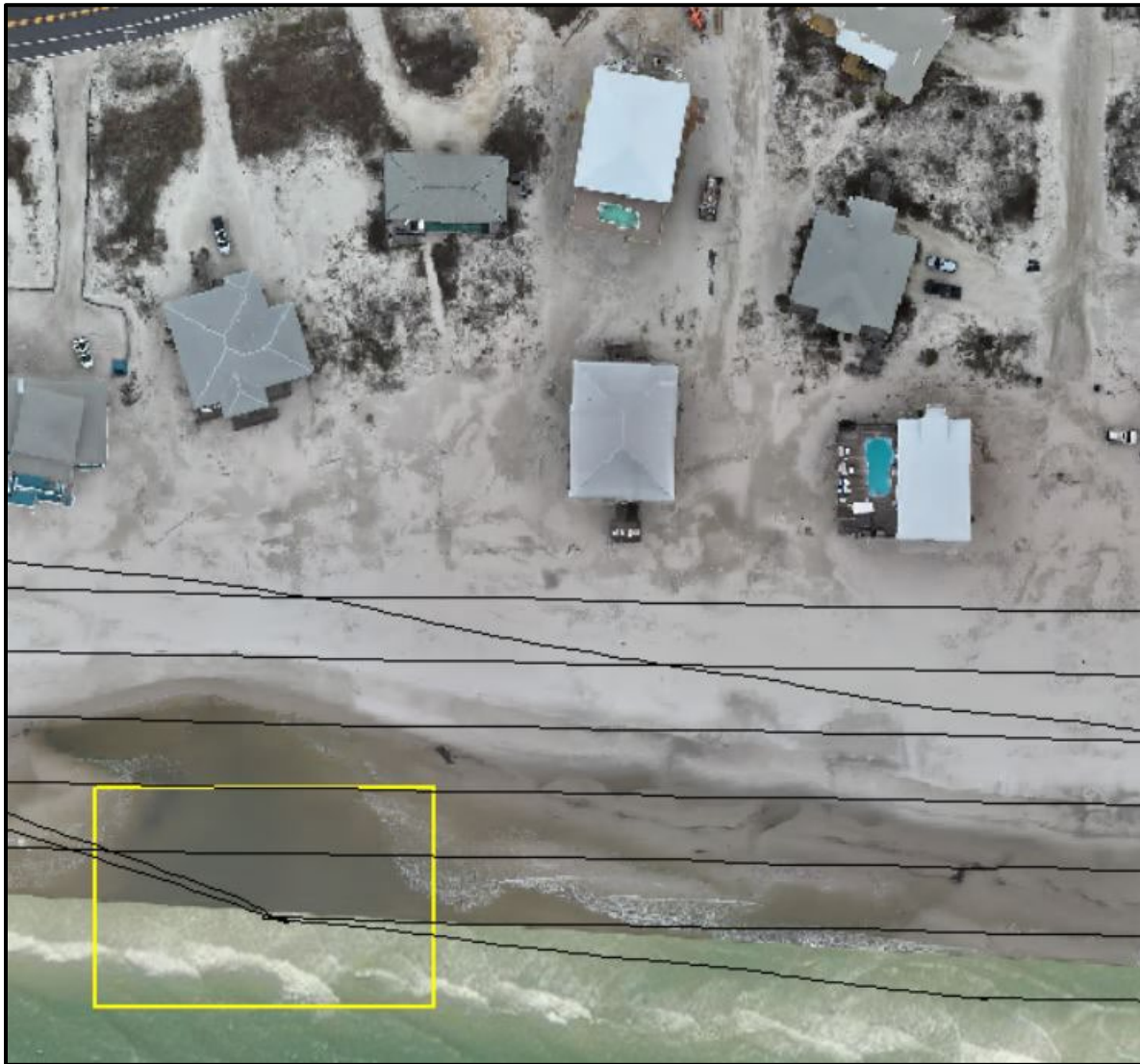
Figure 25. Aerial view of drone transects with highlighted anomaly as an artifact of the drone repositioning.
