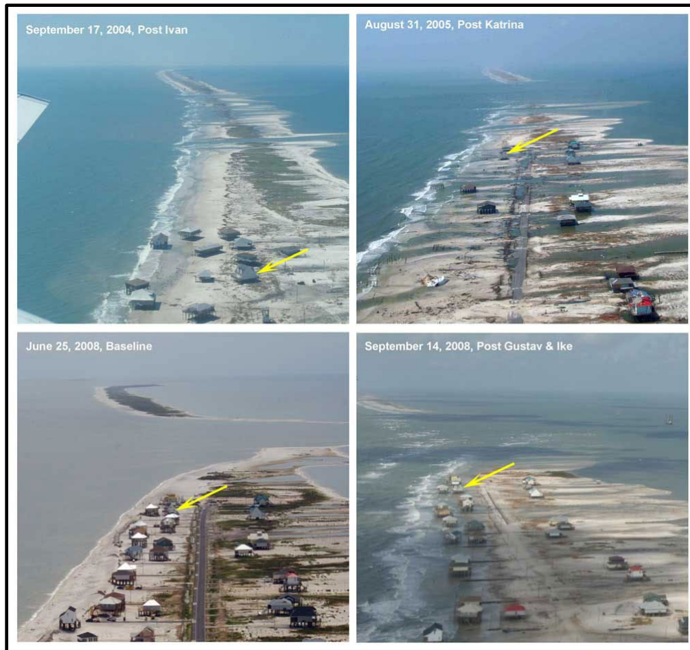
Figure 17. United States Geological Survey images showing the effects of wave erosion on the west end of Dauphin Island after recent hurricanes. The yellow arrows point to the coastline change in relation to a single house (USGS 2022).
