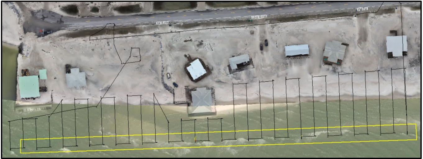
Figure 30. Aerial view showing transect coverage with highlighted area for further analysis. Small hits in the data at the end of the transects are an artifact of the drone repositioning and turning the sensor in the magnetic field.
