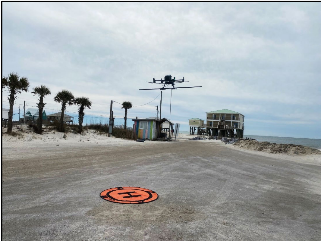
Figure 24. MagDrone R4 takes flight on the West End of the survey area.
