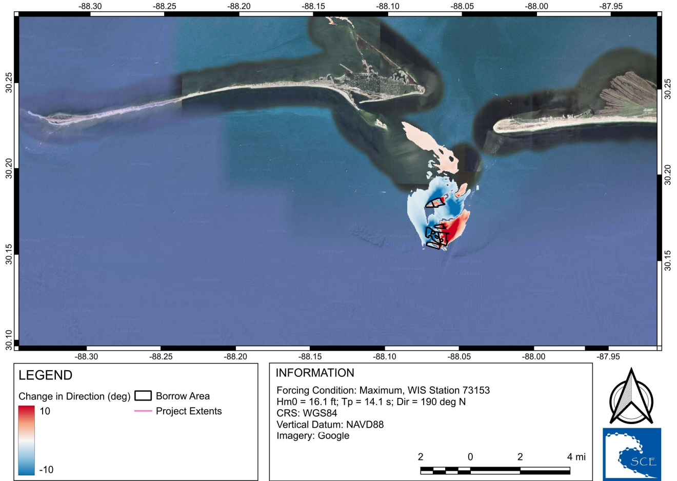
Figure 16. Change in the maximum wave direction (proposed - existing) in degrees. Directional changes between -1 and +1 degree are set transparent.
