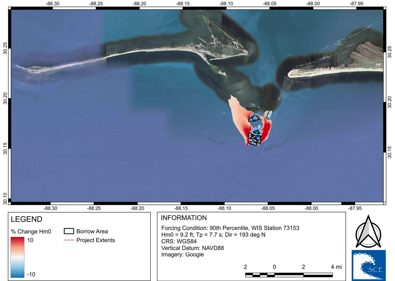
Figure 11. Percent change in the 90 th percentile spectrally significant wave height. Values between -2 and +2 percent are set transparent.
