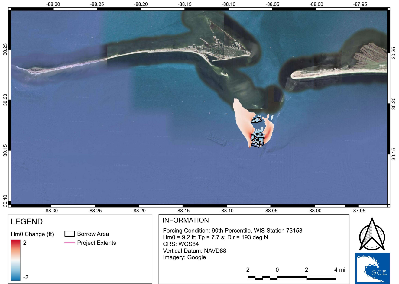
Figure 10. Change in the 90 th percentile spectrally significant wave height (proposed – existing). Values between -0.2 and +0.2 feet are set transparent.
