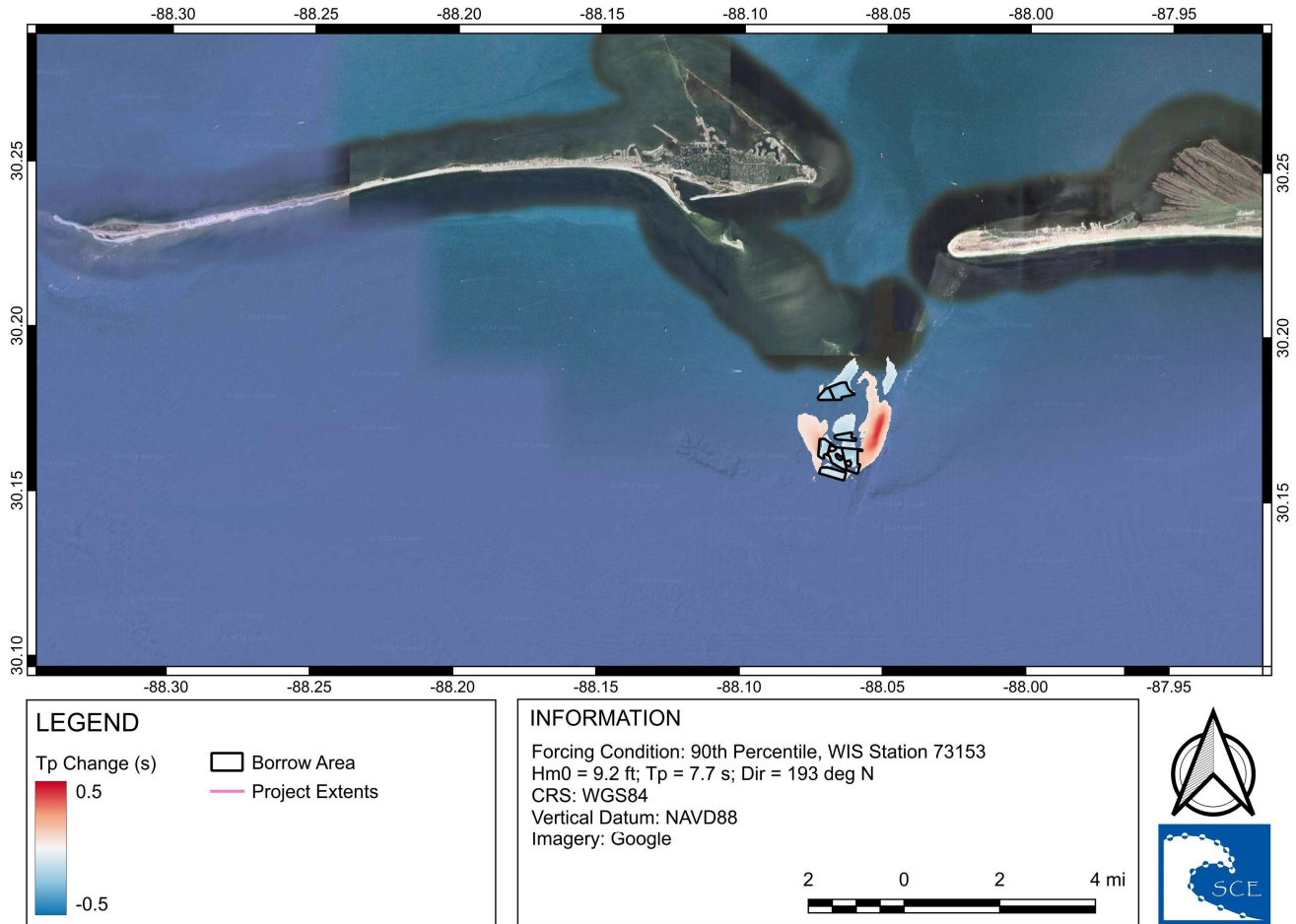
Figure 13. Change in the 90 th percentile wave period (proposed - existing). Changes between -0.05 and +0.05 seconds are set transparent.
